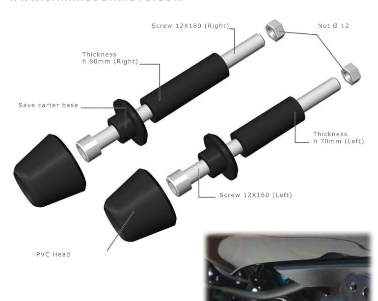
SEARCH AND FIND THE FIXING POINT ON THE MOTOR-BIKE BEFORE START TO MOUNTAIN, USE THE SPECIF-IC THICKNESS AND BOLTS LIKE DESCRIBED IN THE PICTURE (SO YOU CAN GET THE RIGHT PROMINENCE FROM THE MOTORBIKE).
